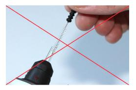
If the probe tip is clogged or the probe is damaged, only MAICO can repair the parts. If you have questions about service or maintenance, please contact:
