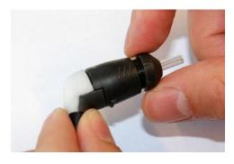
Insert the blue end of the floss from back to front through one of the probe channels. Pull the floss along ist entire length through the channel.
