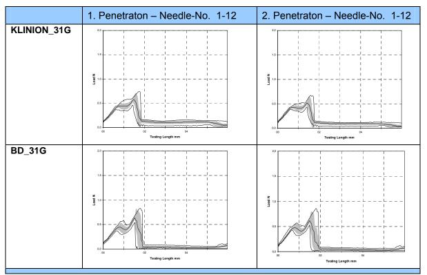
Table 5-4: Comparison of the penetration forces of the 1st and the 2nd penetration
