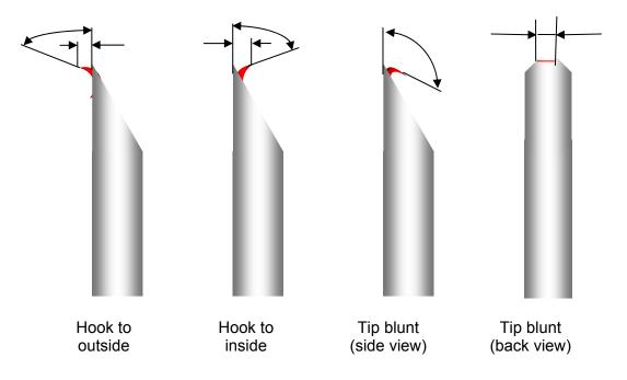
Figure 5-1: Tip defects
