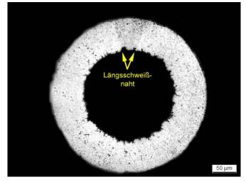
Figure 5-13: BD\_29G - Overview, etched, longitudinal weld
