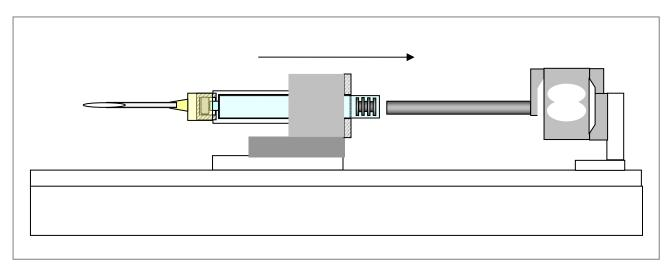
Figure 4-2: Testing Arrangement of plunger force tests (Application Forces, ISO 11608)
