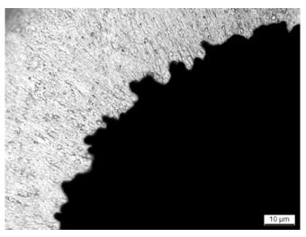
Figure 5-17: KLINON\_31G - Internal surface, wide die marks up to 7 µm depth
