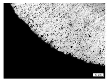
Figure 5-21: BD\_31G - Outer surface, die marks up to 7  $\mu m$  depth
