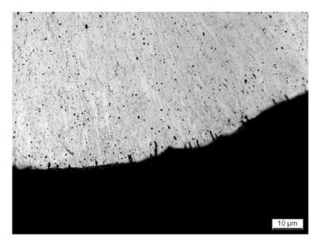
Figure 5-15: BD\_29G – Outer surface, die marks up to 5 µm depth
