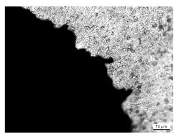
Figure 5-11: KLINON\_29G – Internal surface, wide die marks up to 12 µm depth
