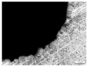
Figure 5-20: BD\_31G - Internal surface, folds up to  $\,$  8  $\mu m$  depth
