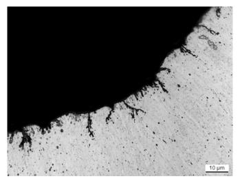
Figure 5-14 BD\_29G - Internal surface, folds up to 12 µm depth
